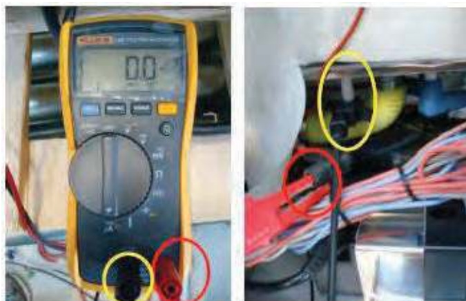
Figure 21 Multimeter connection to the flame control plug
